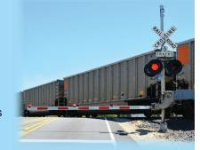
A single, empty boxcar weighs roughly 80,000 pounds (equal to a big rig packed to the gills); one diesel locomotive tips the scales at 200,000 to 400,000 pounds. At 55 mph, a 100-car train needs at least a mile to stop completely — with full emergency braking. The physics doesn't bode well for a car driver.
